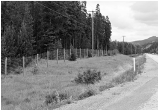
Figure 22. A section of the eight-foot wildlife fence along the Coquihalla Highway. The barrier has been very successful in reducing collisions with big game animals by keeping them off of the highway right-of-way. Photo by Dennis A. Demarchi, north of the Coquihalla Summit, BC, June 2015.
